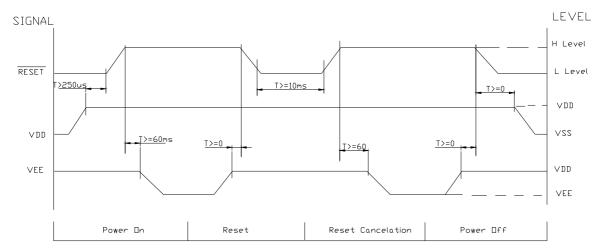
Please maintain the above sequence when turning on and off the power supply of the module.
